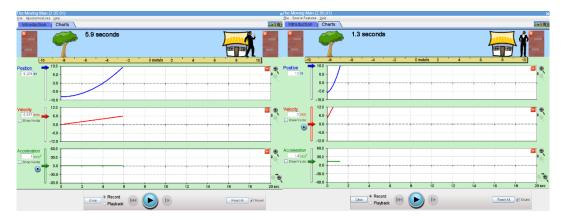
Comparison Three: Compare the graphs of a small acceleration trial and a large acceleration trial.
