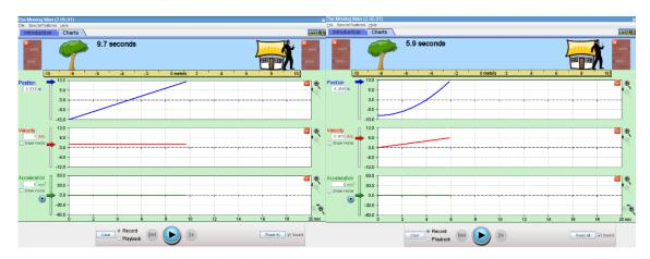
Comparison One: Compare the graphs of a zero-acceleration trial to a positive acceleration trial.
